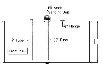
Please note: All sizes are NPTF unless otherwise noted and reference all measurements from the lateral weld seam and the end cap weld seam to the center of the fittings.
